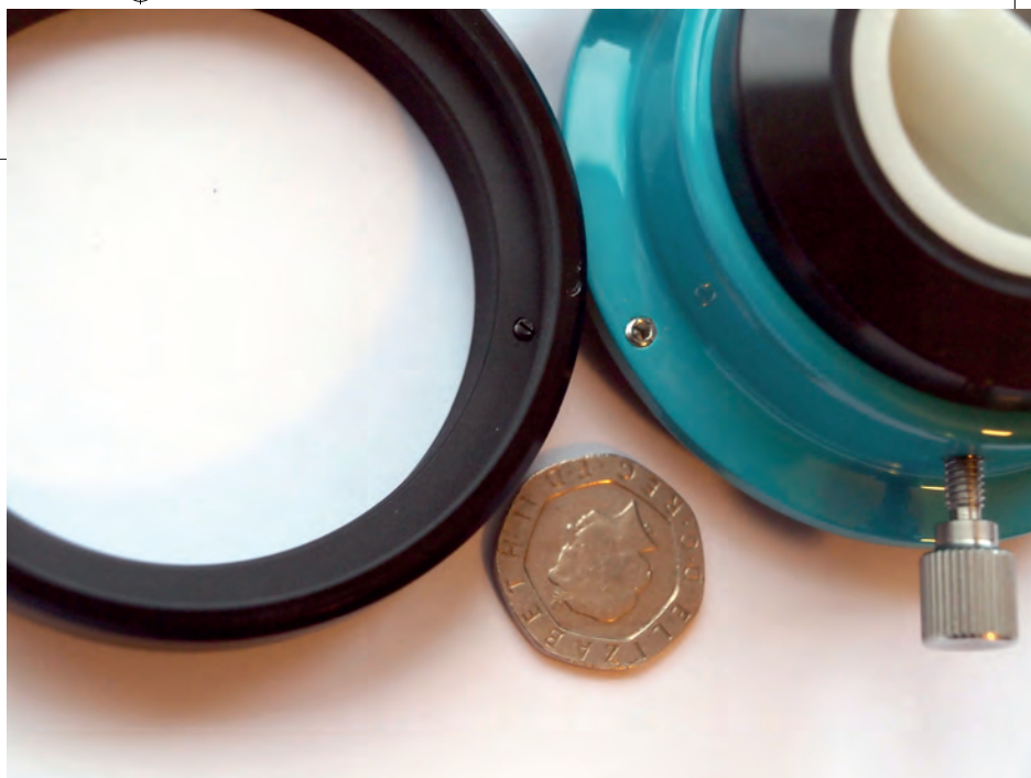
▲ Close up of the tiny flat-head and Allen-key grub screws used in removing the optical back for deployment of the 1.0 \times field flattener.
