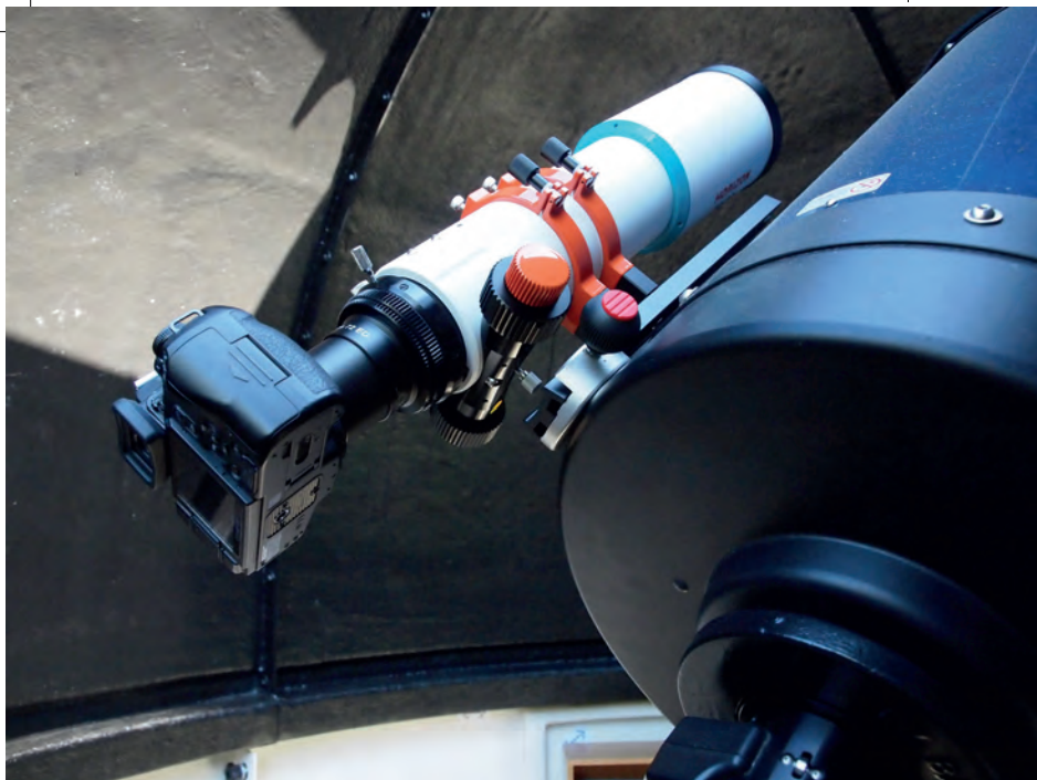
▲ The RVO 72mm ED in its imaging configuration, with a 1.0× field flattener and a DSLR attached, all flying on the coat-tails of the author's 355mm (14-inch) LX200.
