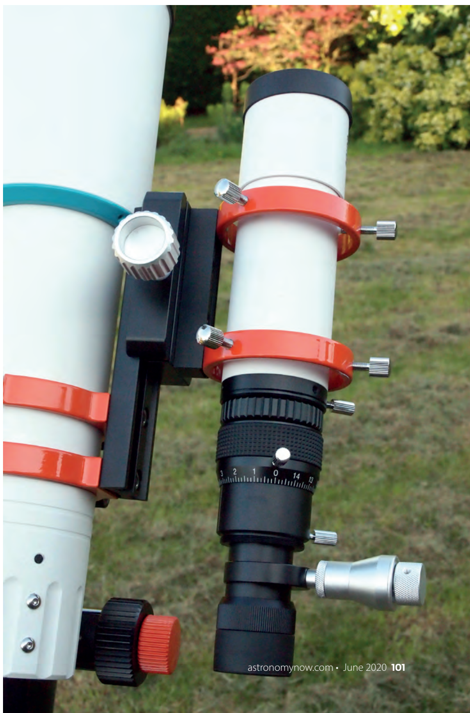
▼ A view of the RVO Horizon 50mm guidescope, showing the indexed helical focuser and 24mm illuminated crosshair eyepiece.
