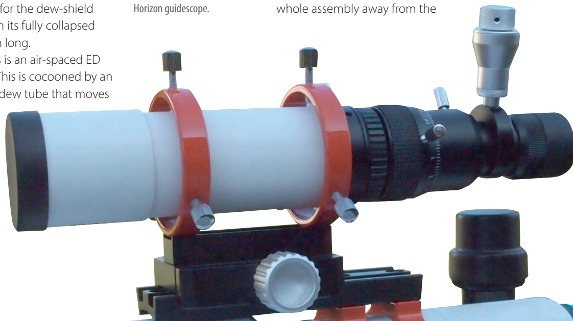
▼ A close up of the three-stage attachment of the 50mm RVO Horizon guidescope.
